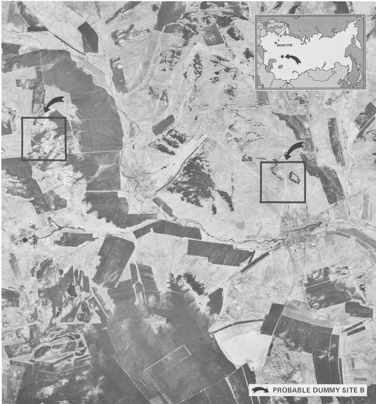
Improvements to CORONA cameras made it possible by November 1967 to discover in KH-4A imagery probable dummy Type-IIIC single silos at Kartaly ICBM Complex southeast of Moscow.
